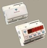
Batching system weighing indicator provides digital or isolated analog output signal for tank/bin/hopper weighing systems. High level serial communication is available in RS232, or RS485 format with Modbus RTU or Profibus protocol. Up to 32 transmitters can be connected point-to-point.
